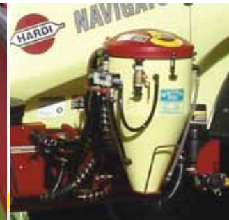
Granni Pot With vortex mixing action for safe, easy transfer chemicals
