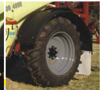
Mudguards Protects nozzles & sprayer from external dirt ingress in transport
