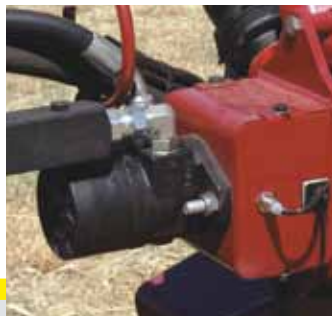
Hydraulic drive Ideal alternative to PTO shaft
